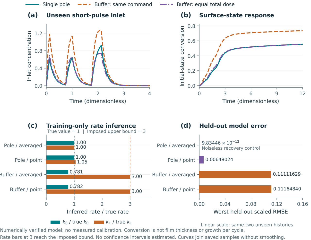
Figure 1 | Delivery and observation effects in a synthetic ALD model. (a) Instantaneous inlet histories. (b) Initial surface-state conversion. (c) Inferred rate multipliers; the reference is 1 and the imposed upper bound is 3. (d) Worst scaled RMSE across two held-out histories on a linear axis. All fitted delivery models are single-pole models. Channel weights are numerical scales, not measured noise. The original four-panel figure is reproduced without changing its data. Conversion is not thickness or growth per cycle.
